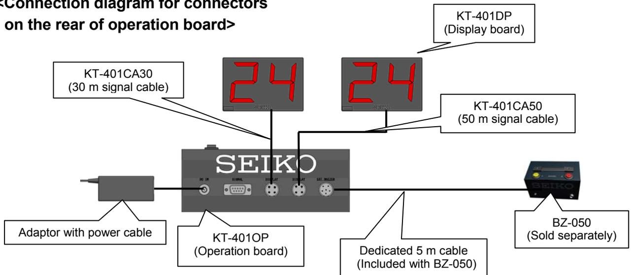
\* 30 m and 50 m signal cables can be connected interchangeably to either of the connectors of the display board.
