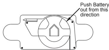
Fig.6b Battery Compartment
